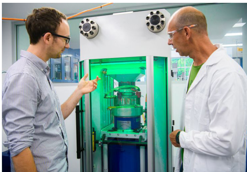
Michael Förster and Slava Shcheka (Lab manager) running a high-pressure experiment on the rapid-quench piston-cylinder apparatus (photo Morris McLennan)
